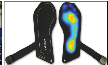
Figure 6. XSENSOR pressure distribution insoles (XSENSOR® Technology Corporation, AB, Canada)
